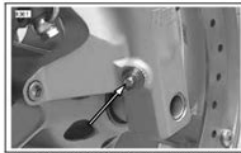
Figure 1-33. Front Fork Compression Damping Adjuster
